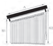
Inclinada cabezal inclinado Sloping blind with sloping covering Inclinée, tête incliné
